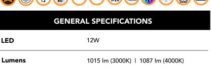
3000K, Warm White 4000K, Cool White Efficacy 84 lm/w (3000K) | 90 lm/w (4000K) 36° | 60° Beam Material Powder Coat Aluminium CRI 92+ Finish White | Black
